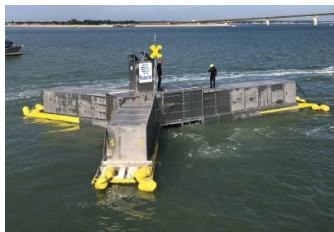
oscillating water column
